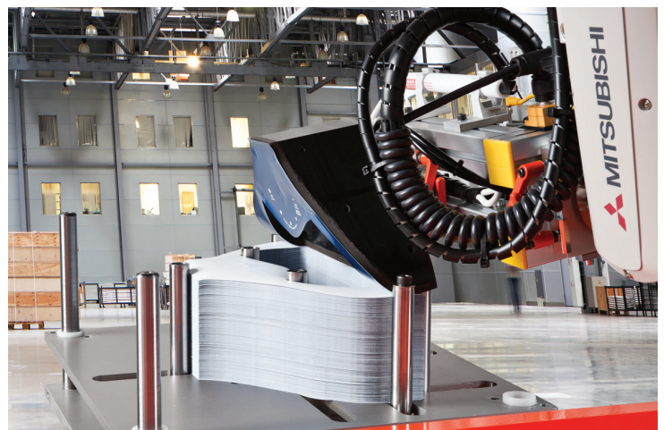
Customized tooling allows you to apply labels and pick parts out of the mold with the same equipment.
